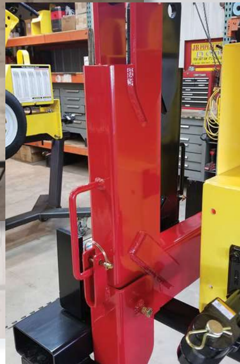
J-Hook mounted for transportation.
